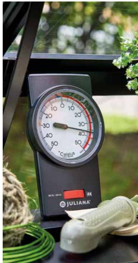
Minimum-maximum thermometer Besides the current temperature, markers show how cold and hot it has been since the last reading. F04355
